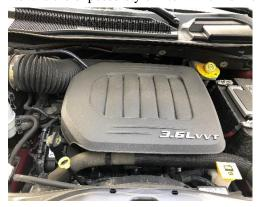
Often, they're accessible in the engine bay rather then under the vehicle. With modern cars utilizing plastic so much, you may need to remove the decorative plastic cover from the engine. These generally just pop out of place without any tools and simply clip back in place. Pictured on the right is the engine with the cover
