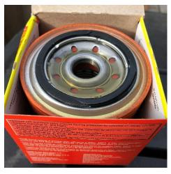
unnecessary wear on critical components. Also, a dab of oil around the new gasket makes hand tightening a little easier.
